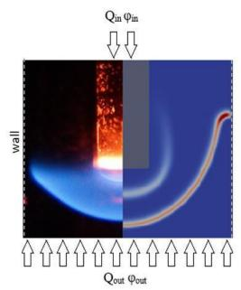
Figure 1. Experimental photo and numerical result on heat release demonstrating cup-like flame and diffusion flame typical for two layered flame structure ( $Q_{in}$ =0.005 1/min,  $\phi_{in}$ = $\infty$ ,  $Q_{out}$ =5.9 1/min,  $\phi_{out}$ =0.7)
