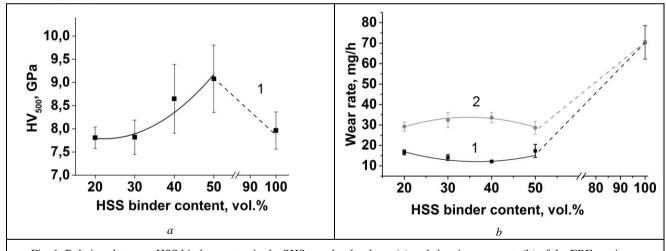
Fig. 1. Relations between HSS binder content in the SHS powder, hardness (a) and abrasive wear rate (b) of the EBF coatings.
